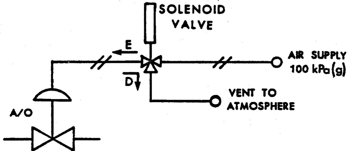
Figure 25: ON/OFF Application of a Solenoid Valve.
