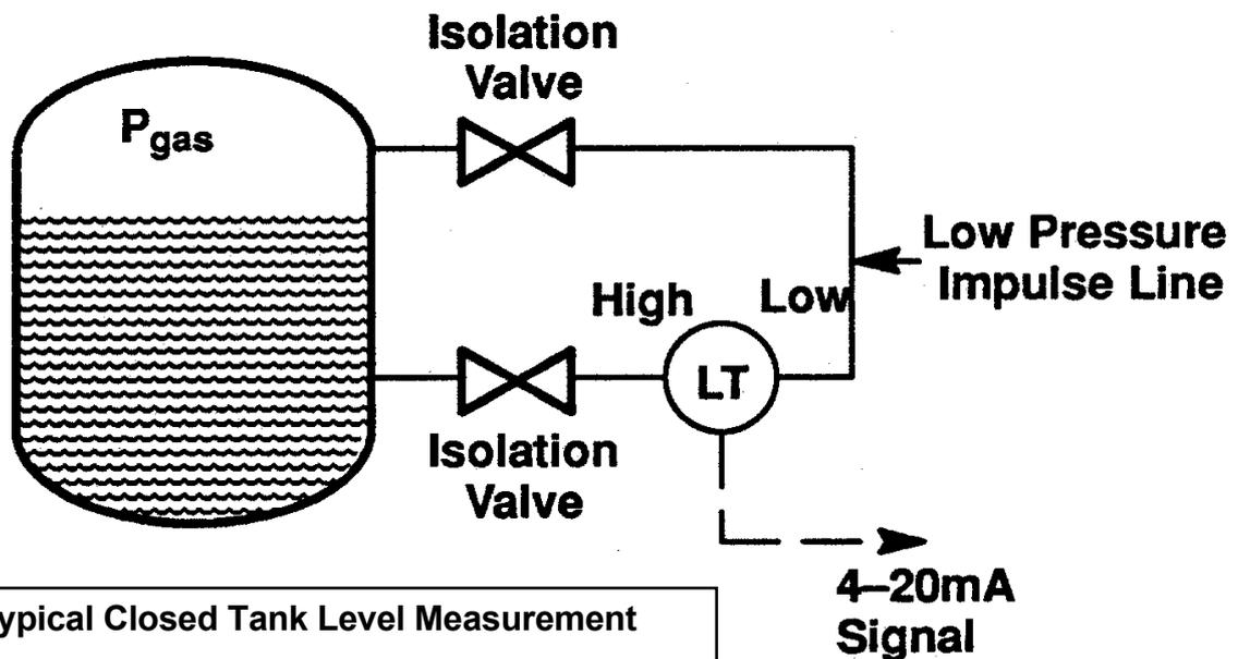
Figure 2: Typical Closed Tank Level Measurement
