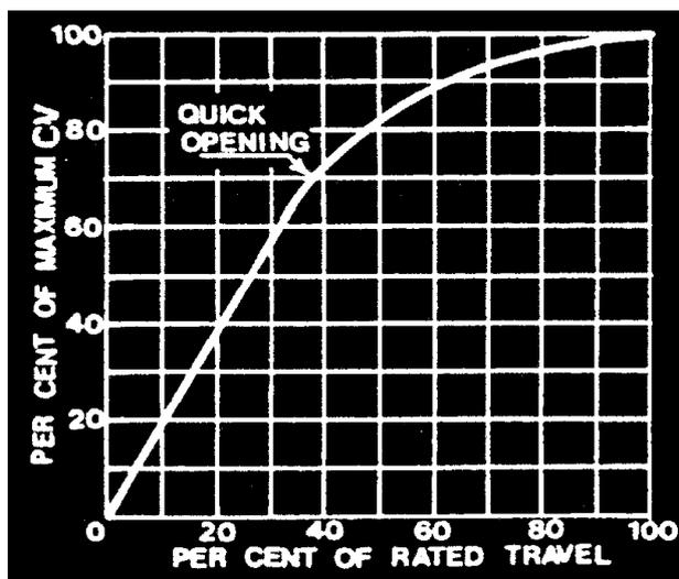
Figure 8(b) Flow Characteristic of Quick Opening Valves
