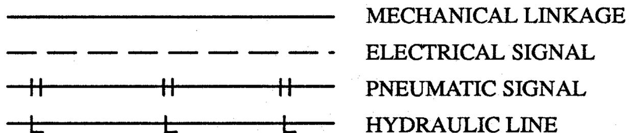
Figure 1. Symbols for Signal Transmission Lines
