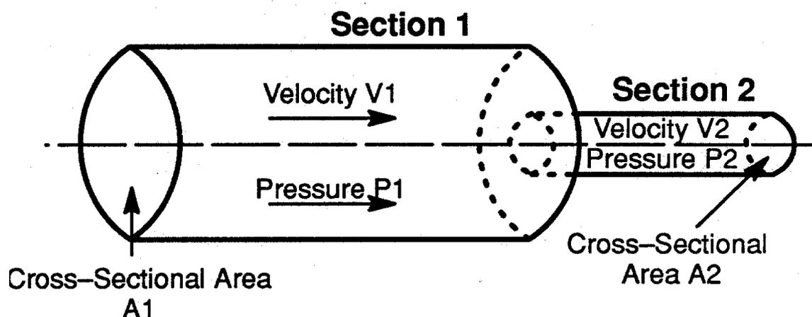
Figure 1. Flow in a Pipe with a Restriction
