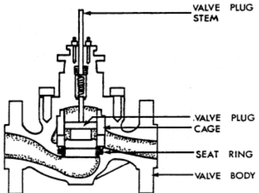
Figure 7: Valve Trim Components For a Globe Valve.
