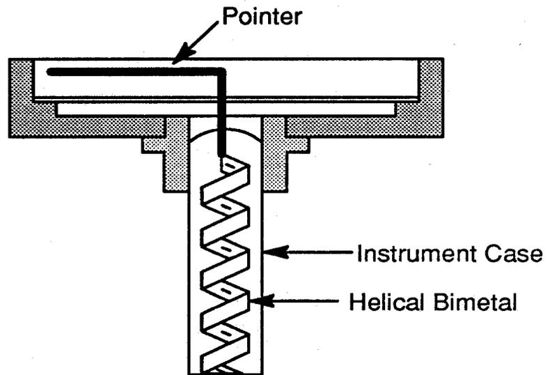
**Figure 2: A Helical Bimetallic Thermometer**
