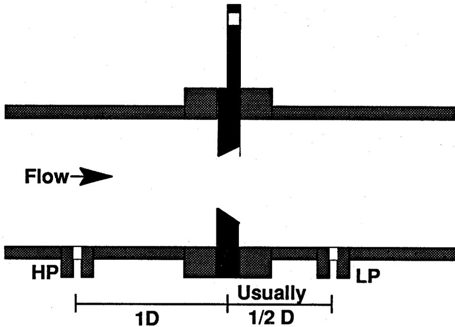
Figure 6: Orifice Plate with Vena Contracta
