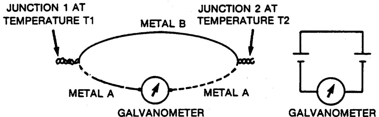
**Figure 3: Thermocouple Circuit.**
