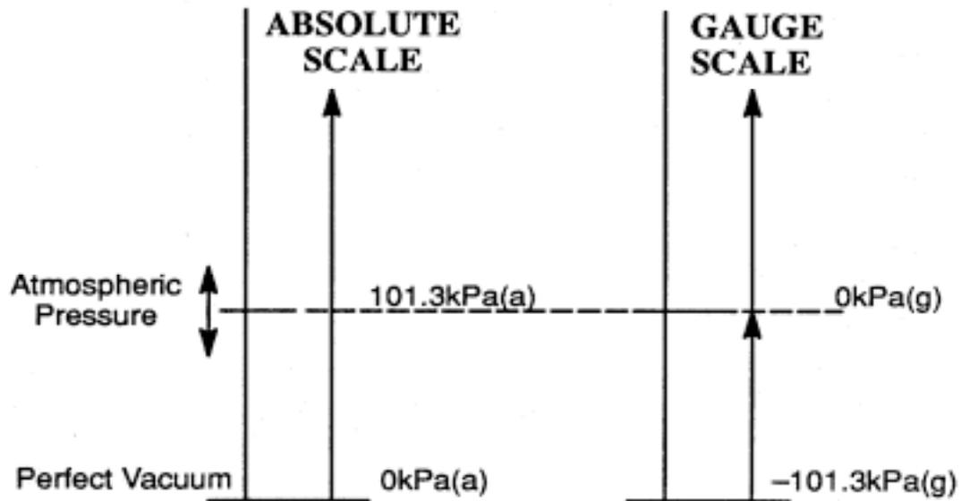
Figure 1: Relationship Between Absolute and Gauge Pressures.
