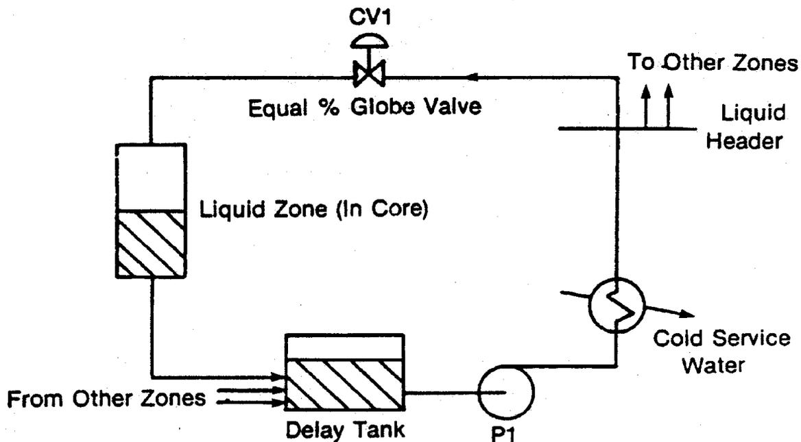
Figure 14: A Simplified Zone Level Control Circuit.
