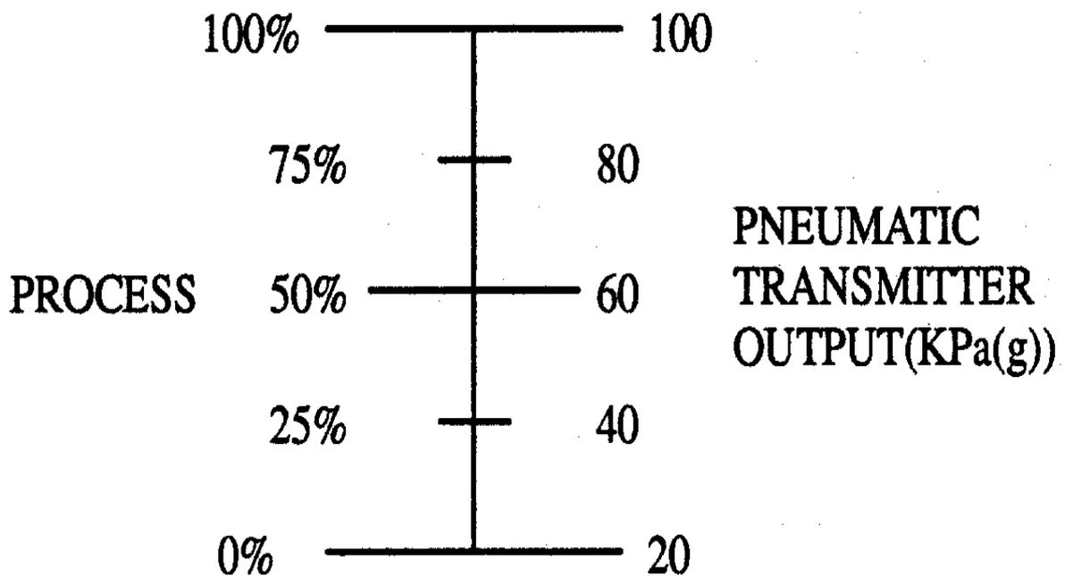
Figure 2. Pneumatic Signal vs Percent Process
