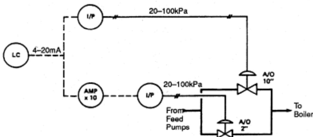
Figure 26. Typical Large/Small Control Valve Installation
