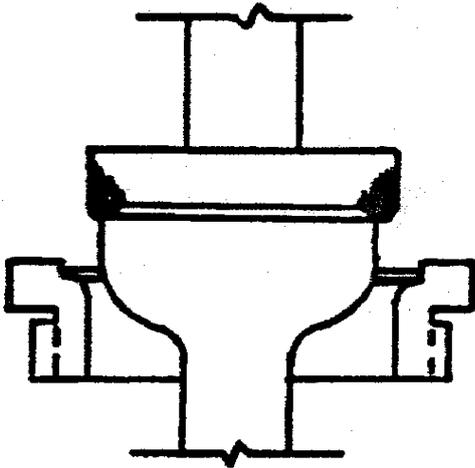
Figure 12(a): A Typical Equal Percentage Valve Plug
