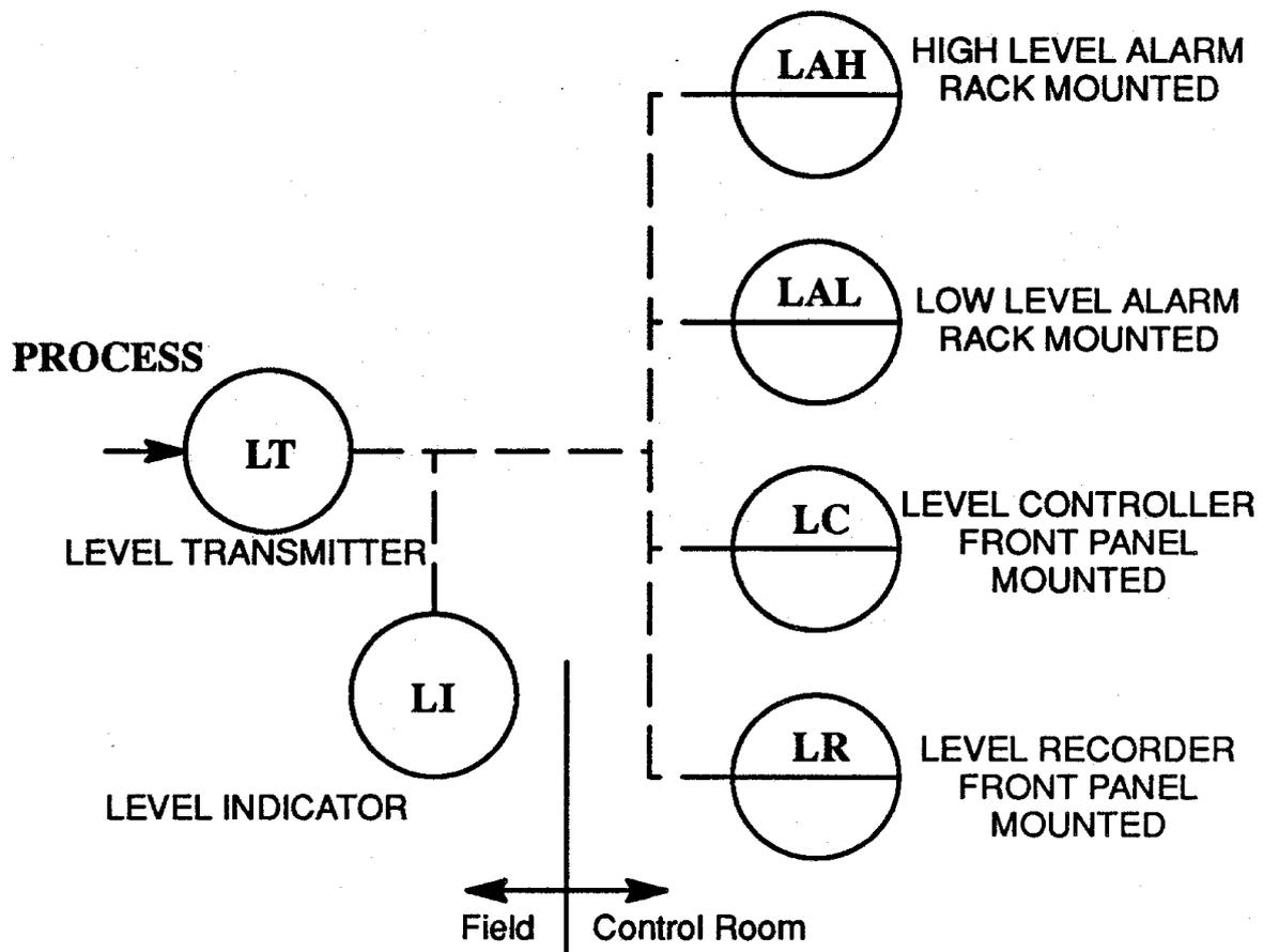
**Figure 3. ISA Symbols Representation of a level Loop**
