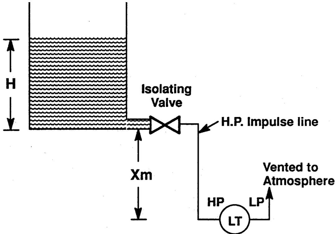
**Figure 6: Level Transmitter with Zero Suppression.**
