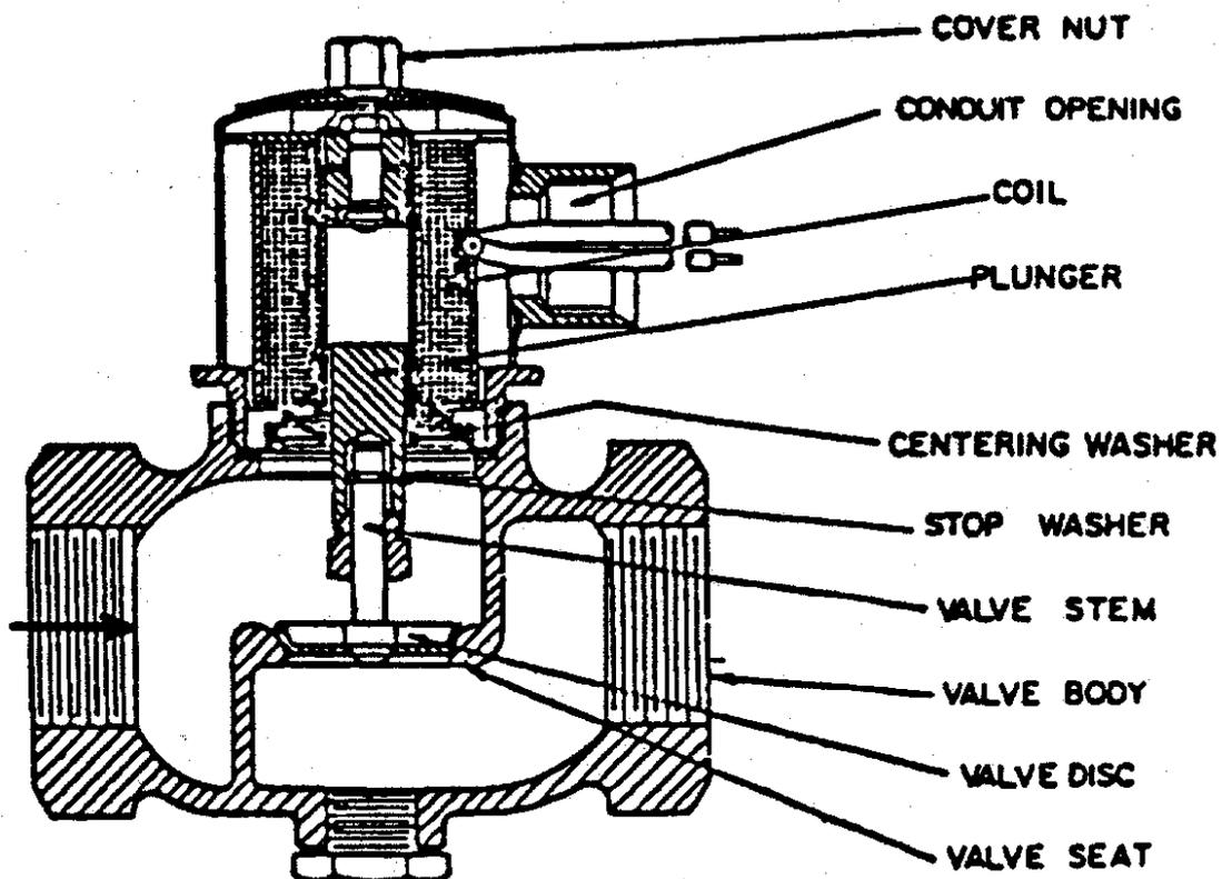
Figure 23: A Two-Way Solenoid Valve.
