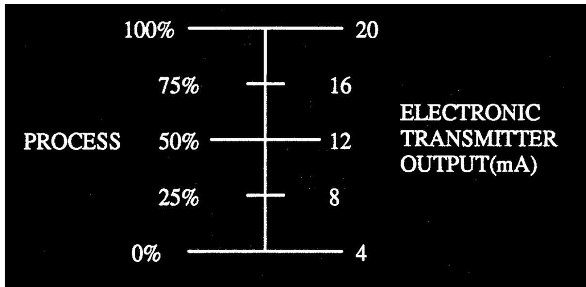
Figure 3. Electronic Signal Values vs Percent Process Measurement
