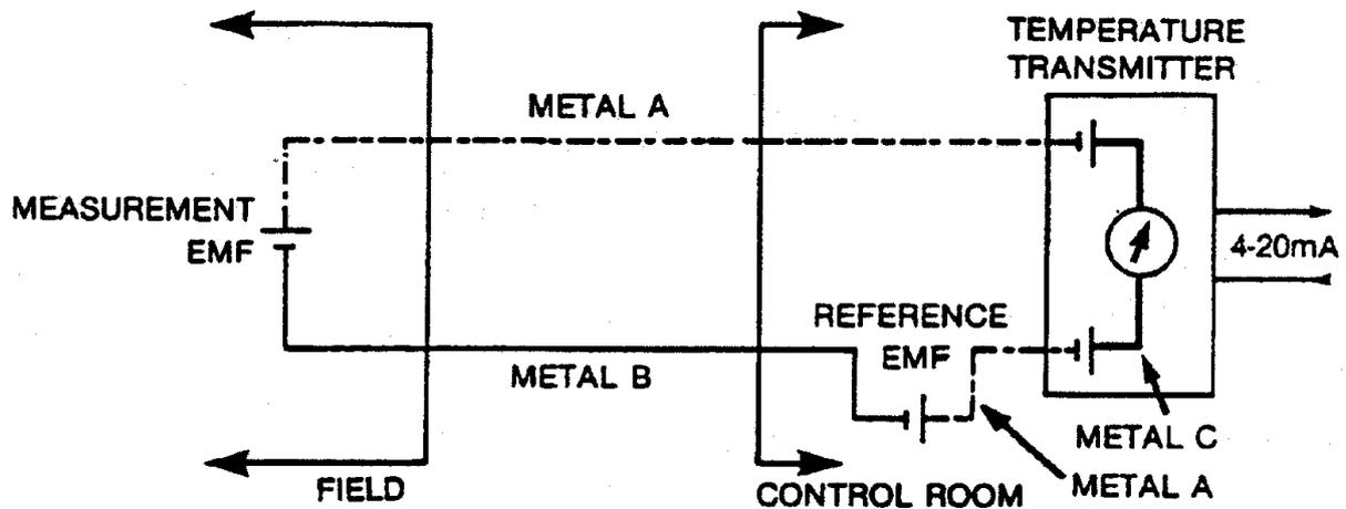
**Figure 5: Equivalent Thermocouple Temperature Transmitter Circuit Diagram.**
